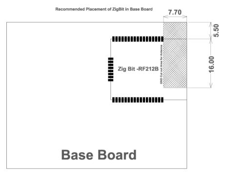
The ZigBit's location and orientation on the carrier board is illustrated in the above Mounting information drawing. The Recommended placement of ZigBit on Carrier Board needs to be accurately followed to ensure performance on the end application.
