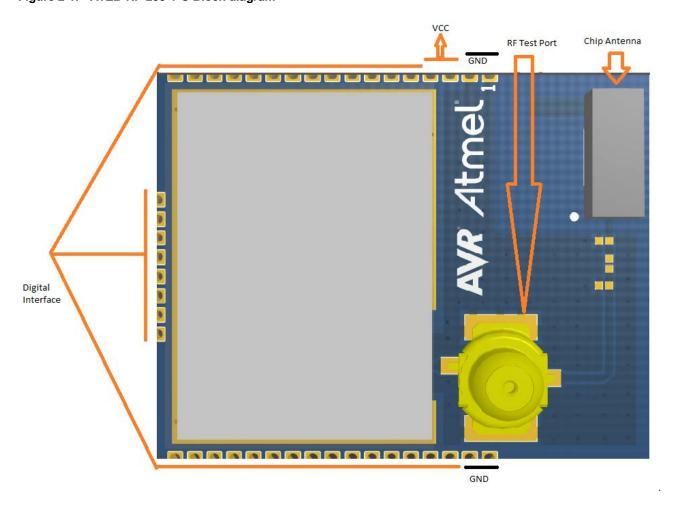
This ZigBit module contains Atmel's AT86RF233 2.4GHz ISM band Transceiver for ZigBee and IEEE 802.15.4 [1].
