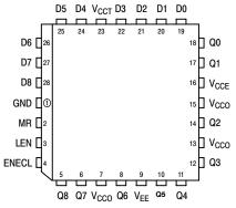
Figure 1. PLCC-28 Pinout (Top View)
