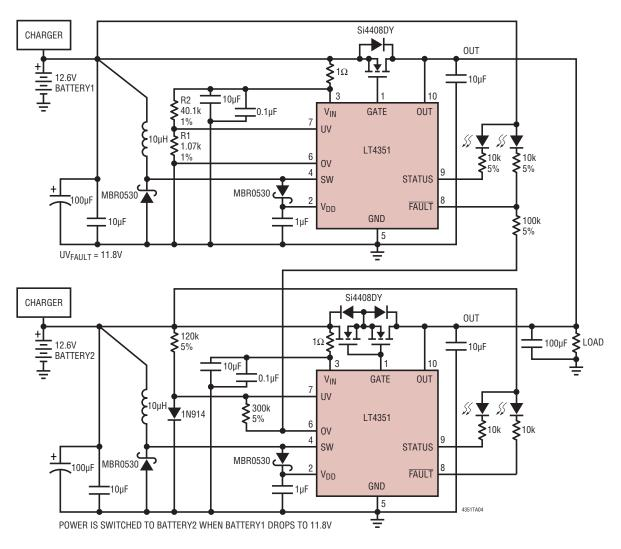
Primary Battery with Secondary Battery Backup
