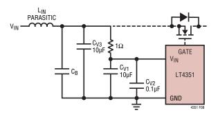
Figure 8. V<sub>IN</sub> Capacitors
