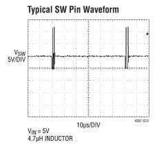
SW Pin Waveform at Maximum Boost Regulator Output
