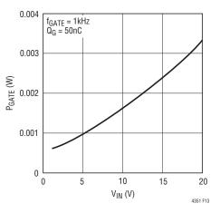
Figure 13.  $P_{GATE}$  vs  $V_{IN}$  ( $V_{DD} = V_{IN} + 10.7$ )
