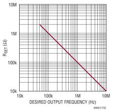
Figure 2. R<sub>SET</sub> vs Desired Output Frequency
