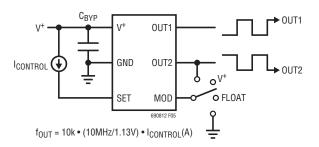
Figure 5. Current Controlled Oscillator
