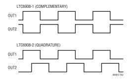
Figure 3. Output Waveforms for LTC6908-1, LTC6908-2
