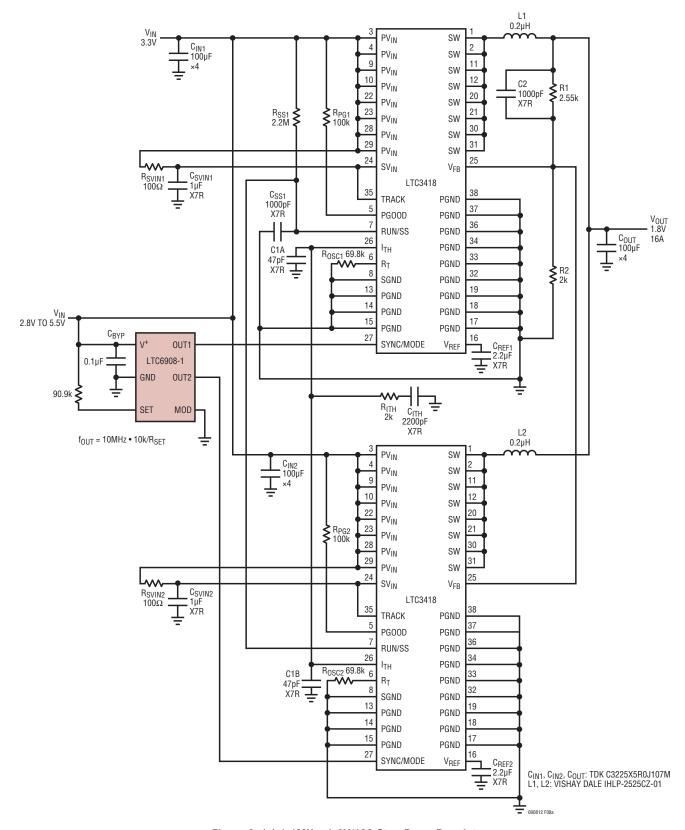
Figure 8. (a) 1.1MHz, 1.8V/16A Step-Down Regulator
