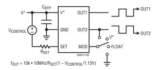
Figure 6. Voltage Controlled Oscillator
