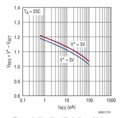
Figure 1. V+ - V<sub>SET</sub> Variation with I<sub>RES</sub>
