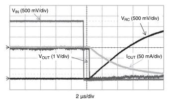
$V_{IN} = 2.8~V,~R_{LOAD} = 18~\Omega,~L_{LOAD} = 80~\mu H$  Input Falling Edge Triggering Operation
