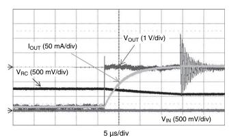
$V_{IN}$  = 2.8 V,  $R_{LOAD}$  = 18  $\Omega$ ,  $L_{LOAD}$  = 80  $\mu H$ Inductive Discharge OUT2 to OUT1
