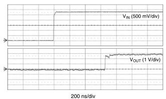
$V_{IN} = 2.8 \text{ V}, \ R_{LOAD} = 18 \ \Omega, \ L_{LOAD} = 80 \ \mu\text{H}$  Input Rising Edge Trigger Response Time
