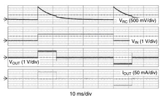
$V_{IN}$  = 2.8 V,  $R_{LOAD}$  = 18  $\Omega$ ,  $L_{LOAD}$  = 80  $\mu H$ Steady State Operation
