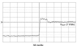
$V_{IN}$  = 2.8 V,  $R_{LOAD}$  = 18  $\Omega$ ,  $L_{LOAD}$  = 80  $\mu$ H
