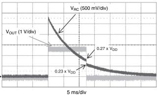
$V_{IN}$  = 2.8 V,  $R_{LOAD}$  = 18  $\Omega$ ,  $L_{LOAD}$  = 80  $\mu H$  RC Threshold Voltage
