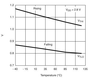
IN Threshold Voltage vs. Temperature
