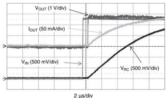
$V_{IN} = 2.8~V,~R_{LOAD} = 18~\Omega,~L_{LOAD} = 80~\mu H$  Input Rising Edge Triggering Operation
