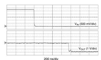
$V_{IN} = 2.8 \text{ V}, \text{ R}_{LOAD} = 18 \ \Omega, \text{ L}_{LOAD} = 80 \ \mu\text{H}$  Input Falling Edge Trigger Response Time
