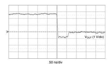
$V_{IN}$  = 2.8 V,  $R_{LOAD}$  = 18 Ω,  $L_{LOAD}$  = 80 μH Falling Edge  $T_{BBM}$
