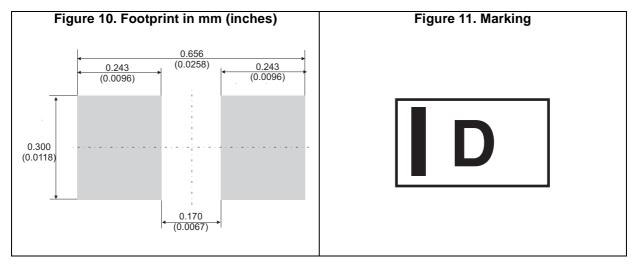
The marking codes can be rotated by 90° or 180° to differentiate assembly location. In no Note: case should this product marking be used to orient the component for its placement on a PCB. Only pin 1 mark is to be used for this purpose.
