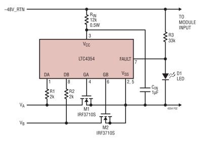
Figure 2. -36V to -72V/5A Design Example
