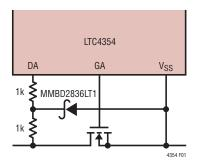
Figure 1. Method of Protecting the DA and DB Pins from Negative Inputs. One Channel Shown
