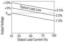
The voltage tolerance envelope shows typical load regulation characteristics for this product series. The tolerance envelope is the maximum output voltage variation due to changes in output loading.
