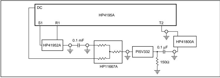
Figure 1. Differential Gain/Phase
